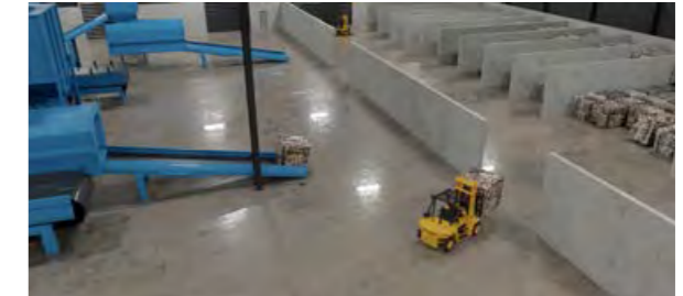
Separated recyclables (paper, cardboard, plastics, glass, aluminium and steel) are stored in bays until they can be transported to various recyclers to be made into new products.
