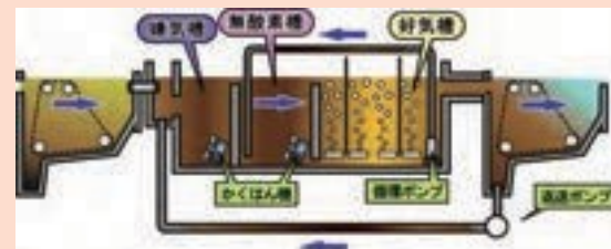
Aerobic tank - Aerobic tank Oxygen-free tanks - water from anaerobic tanks is mixed with water from aerobic tanks by circulation pumps without air.
